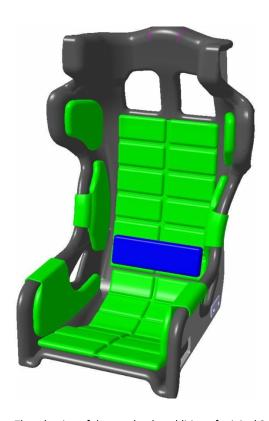
The adaption of the seat by the addition of original **Sabelt** seat padding shown in green and blue in Attachment 12 is permitted. Each padding shape may only be used in the specific and correct location and direction as shown in Attachment 12.
