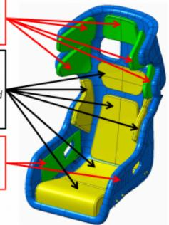
The adaption of the seat by removing or adding of original **Recaro** seat padding is forbidden in the areas of the seat shown in green colour on the illustration above.
